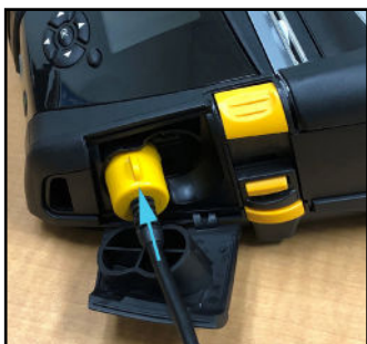
1. Insert connector in communications port.
