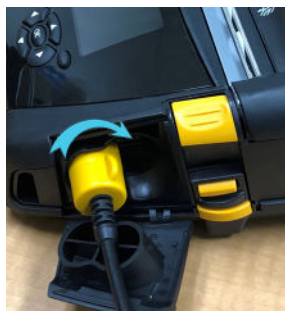
2. Rotate locking cap clockwise to secure.
